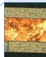
Micrographic image of a trimetal strip cross section
